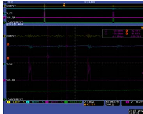
FIGURE 35. ZOOM IN, CH1: OUTPUT VOLTAGE, CH2: VOLTAGE ON C3, CH3: Vds OF Q4_SR, CH4: LOAD CURRENT
