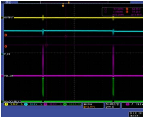
FIGURE 34. SHORT CIRCUIT, CH1: OUTPUT VOLTAGE, CH2: VOLTAGE ON C3, CH3: Vds OF Q4_SR, CH4: LOAD CURRENT
