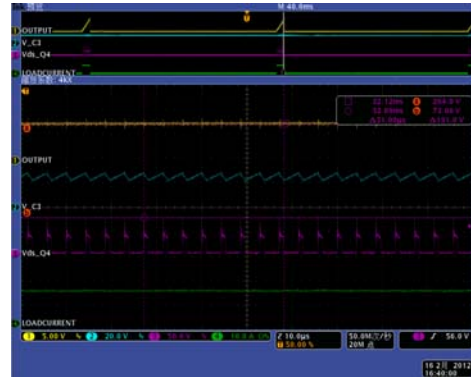
FIGURE 33. ZOOM IN, CH1: OUTPUT VOLTAGE, CH2: VOLTAGE ON C3, CH3: Vds OF Q4_SR, CH4: LOAD CURRENT
