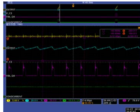
FIGURE 37. ZOOM IN, CH1: OUTPUT VOLTAGE, CH2: VOLTAGE ON C3, CH3: Vds OF Q4_SR, CH4: LOAD CURRENT
